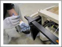
Using a 3/4 SAE socket, 9" extension, and ratchet remove the 4 bolts holding the shipping bed stand onto the head board bracket.
