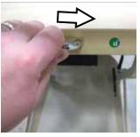
Clamp the footboard bracket slide mechanism by turning both retention knobs clockwise until hand tight.
