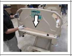
19. Place the footboard into the foot board bracket assembly.
