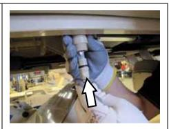
27. If your bed is equipped with the optional pendant, plug it into the available pendant port on either side of the bed. Unscrew cap on pendant port. Align arrows and insert pendant connector into pendant port. Slide up and screw on threaded retaining collar.
