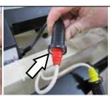
Foot Mounted Actuator Extension Cables (4 pin, DIN style, double keyed connector to 6 pin modular connector) Connects foot mounted actuator cables to CB09 control box. Retainer requires small slot screwdriver to remove (arrow)
