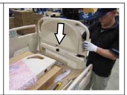
18. Place the headboard into the head board bracket assembly.
