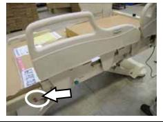
14. On Spirit Select beds there are two shipping pins located behind the foot rail assemblies.
