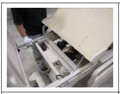
25. Continue to lift the knee/foot hinged connection and gently lay the deck sections back as shown above. The CB10 or CB11 control box is now accessible.
