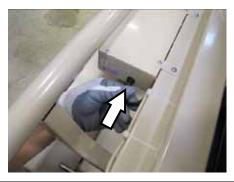
26. Connect the battery cable to the side DC jack of the CB10 or CB11 control box.
