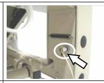
To operate the Nurse Call feature, press the red NURSE button on the rail patient control (inside of each head rail control). This will send a Nurse Call signal to the nurses' station when appropriately connected to the communication system of your healthcare facility.
