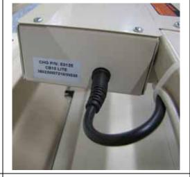
CB10Lite serial number label (affixed to enclosure next to battery connection)
