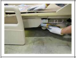
Reach under bed and cut packaging strap wrapped around foot-end leg assembly and the frame.
