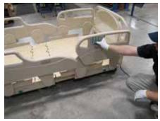
29. Once the bed is fully lowered and all bed motion has automatically stopped CONTINUE to HOLD the BED DOWN button until the two tone audible indicator sounds.
