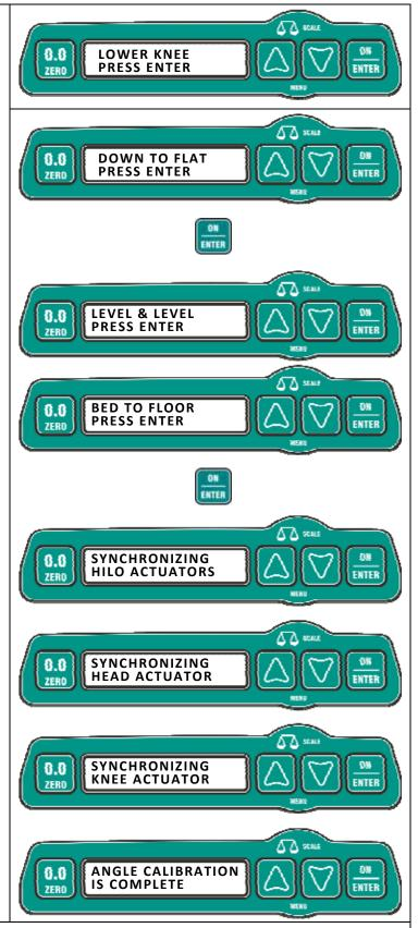
**IMPORTANT:** Because of manufacturing tolerances, the mass of the bed alone may be insufficient to completely compress the Hi-Lo springs. To ensure that the bed is sitting completely flat (the mattress deck is perfectly parallel with floor) when in the lowest position, CHG Hospital Beds recommends that the bed angle is calibrated with at least 60kg (132.2 lbs) on the bed.
