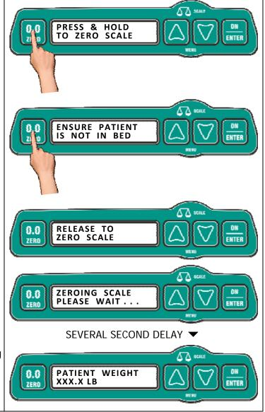
IMPORTANT: The scale cannot be zeroed if the bed has been placed in any Trendelenburg or Reverse Trendelenburg position. Ensure that the bed has been restored to fully horizontal and displaying 0° TREND or revTREND angle before attempting to zero the scale. Refer to page 47 for instructions.
