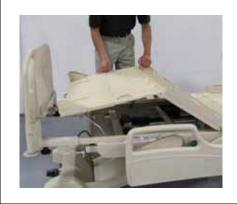
1. Lift the foot and knee sections together until the angle between them is greater than 90°.
