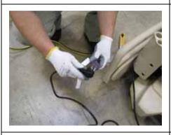
Connect the bed to mains A/C power either directly into the a properly grounded wall outlet or into a suitable extension cord connected to a properly grounded wall outlet.
