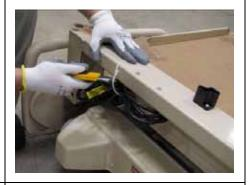
3. Remove the plastic tie wrap around the main power supply cord bundle.
