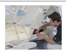
Using a small, slot screw driver, depress the retaining clip on both head siderail control cables and disconnect both cables.
