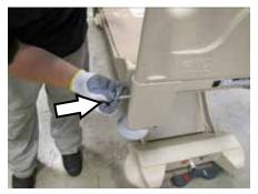
20. Install both foot board lanyard pins into the holes in the foot board bracket.
