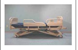
To lower the bed, press the BED DOWN arrow on the footboard staff control, the rail staff controls, or on the pendant.
