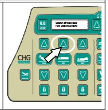
On Spirit Select<sup>™</sup> beds, the factor default setting for obstruction sensors is ENABLED. In the rare event of component failure and/or malfunction, the obstruction sensor system can be disabled in the Service Menu to restore bed functionality until the bed can be properly serviced. Refer to page 89 for instructions.
