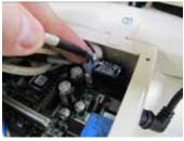
DC Power Cable (Ø5.5 mm X Ø2.5 mm male plug end) Provides 24VDC power from CB09 control box to DC power input header on CB10/CB11 control box
