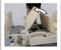
2. Lift the foot section away from the knee section at the hinge, to separate the sections.
