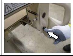
21. Install 4 black plastic barbed clips (from step 17) into the 4 holes it head board bracket that were used to attach the shipping bed stand.
