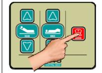
Ensure that the attached "dummy plug" is inserted to an inactive Nurse Call port.
