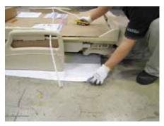
11. If your bed is equipped with the optional obstruction sensors, pull out protective shipping cover installed over the lower leg obstruction sensor. Discard protective shipping cover.
