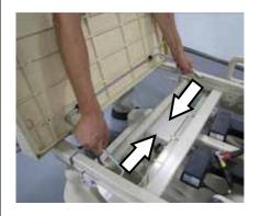
Disengage the foot bail from the frame by flexing the two ends together as shown.
