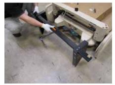
Lift shipping bed stand away from head board bracket. Discard shipping bed stand and fasteners.
