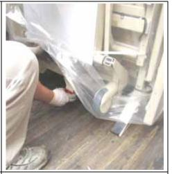
Ensure the brake is engaged before attempting to lower/lift the bed. Attempt to rotate a caster to confirm that the brake has been engaged.
