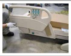
Rotate both head rail assemblies and lock/latch in the UP position. Pull out all packaging tucked in between the rail arms, panel, and bracket. Discard all packaging materials.
